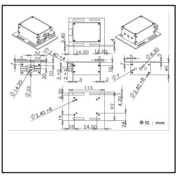
From 200 to 1100nm. Incoming photons generate corresponding electrical pulses which maybe conveniently read out At the TTL output. The gating function allows the module to be disabled between measurements to provide protection Against accidental overload.
