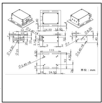
From 1000 to 1700nm. Incoming photons generate corresponding electrical pulses which maybe conveniently read out At the TTL output. The gating function allows the module to be disabled between measurements to provide protection Against accidental overload.
